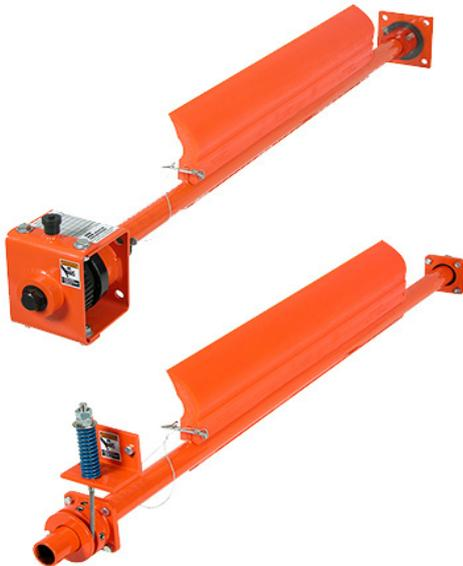
The Martin® PIT VIPER™ Pre-Cleaner was specially developed to simplify blade replacement and to reduce costs. It makes it possible to quickly and easily replace the blade without any tools by removing and reinserting a single retaining pin.
